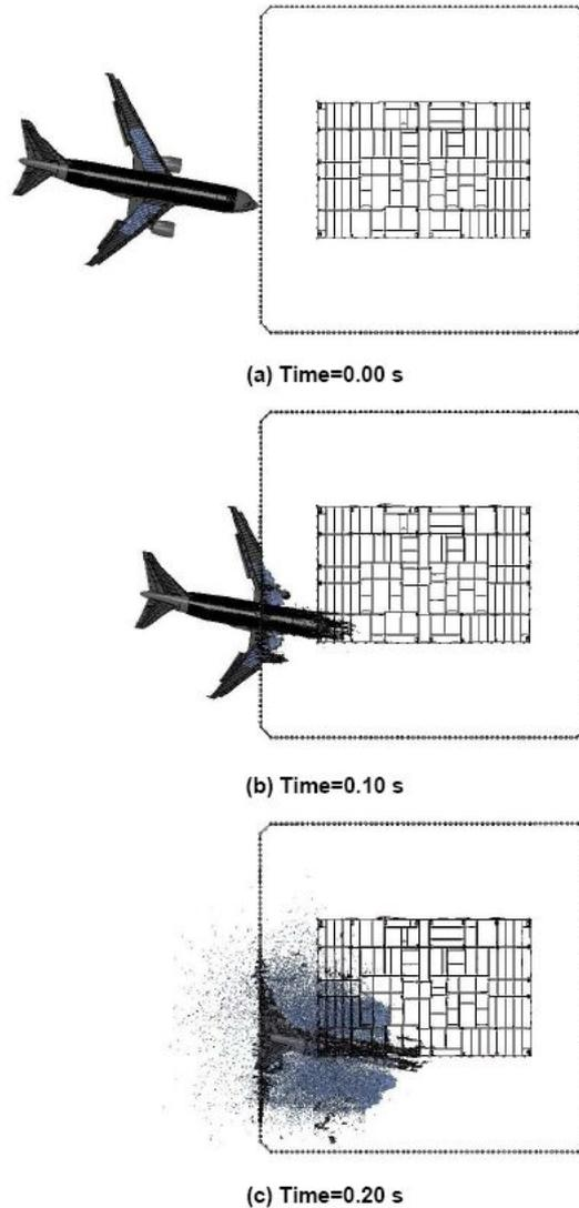
**Figure 7-34. WTC 2 base case global impact analysis (plan view).**
