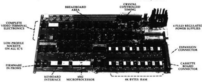
Labels on the diagram include: BREADBOARD AREA, CRYSTAL CONTROLLED TIMING, COMPLETE VIDEO TERMINAL ELECTRONICS, 4 FULLY REGULATED POWER SUPPLIES, LOW-PROFILE SOCKETS ON ALL IC'S, EXPANSION CONNECTOR, FIRMWARE IN PROMS, CASSIETTE BOARD CONNECTOR, KEYBOARD INTERFACE, 6502 MICROPROCESSOR, and 8K BYTES RAM.
